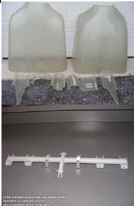
[GP4] Elevator torque tube and pillow blocks fabricated by Raymond Beazley, who is supplying all the metal parts
