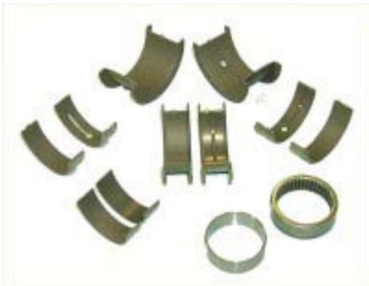
engine that is used in many Beech and Cessna singles and twins as an example. The IO-520 overhaul manual lists the minimum crankshaft bearing clearance as 0.0018 inch at normal room temperature.
