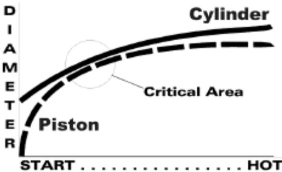
The problem is made worse by the fact that most cylinders barrels are designed with a taper, or "choke" in the top one-third of piston travel. This is done to pre-compensate the barrel for the fact that, as the engine comes up to operating temperature, the top of the cylinder (where the combustion process takes place) is a lot hotter than the bottom of the cylinder, and therefore expands considerably more. If cylinders were perfectly cylindrical at room temperature, then they'd
