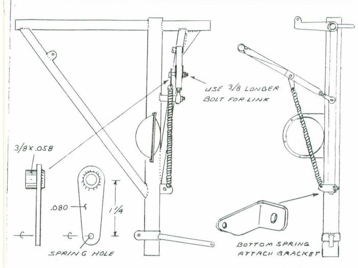
LANDING LITE CAN BE MOVED AFT IF NECESSARY BY USING SPACERS
